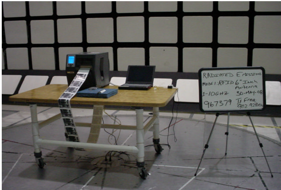
Figure 4 Test setup for Radiated Emissions 1-10GHz Front and Rear View
