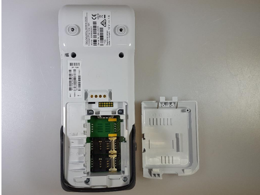
Photo 5: Battery cover removed
