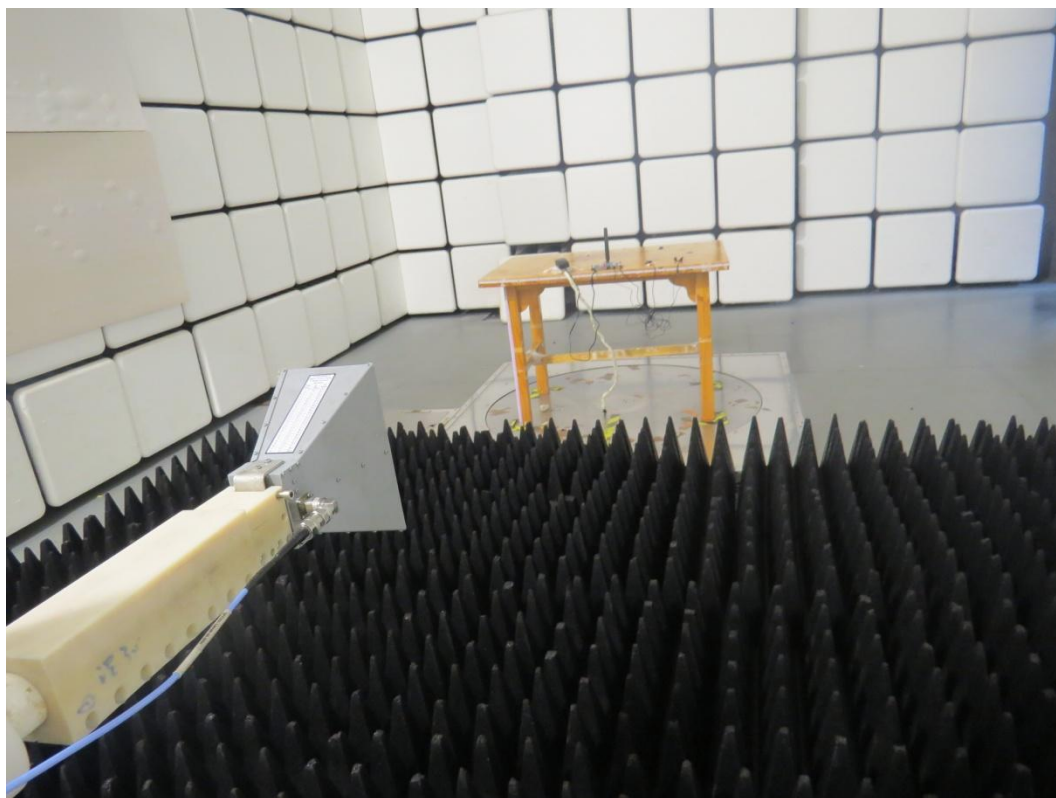
Picture 1 Radiated Emission Test Setup
