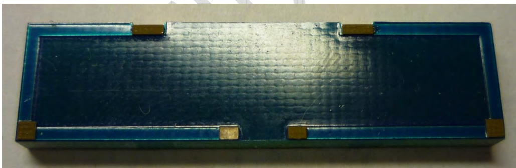
Figure 4 Bottom side of antenna chip showing PCB surface mounting
