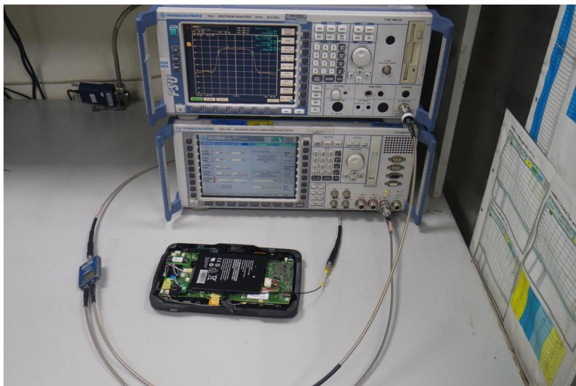
**Radiated Emission Set up Photos****Below 1GHz**
