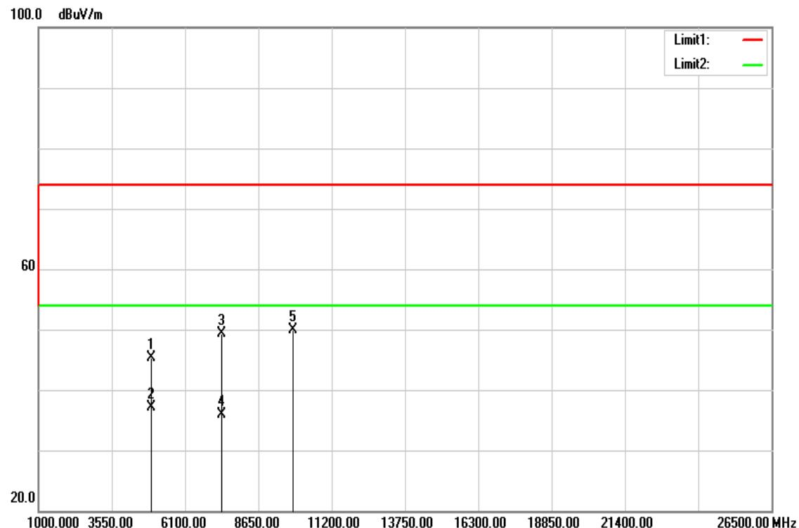
**Operation Mode:** TX / IEEE 802.11b / CH High**Test Date:** October 22, 2016**Temperature:** 27°C**Tested by:** Dennis Li**Humidity:** 53% RH**Polarity:** Ver. / Hor.
