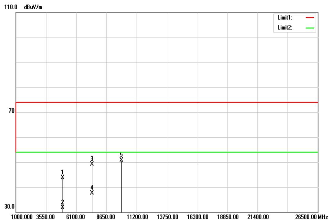
**Operation Mode:** GFSK / TX / CH High**Test Date:** October 25, 2016**Temperature:** 27°C**Tested by:** Dennis Li**Humidity:** 53 % RH**Polarity:** Ver. / Hor.
