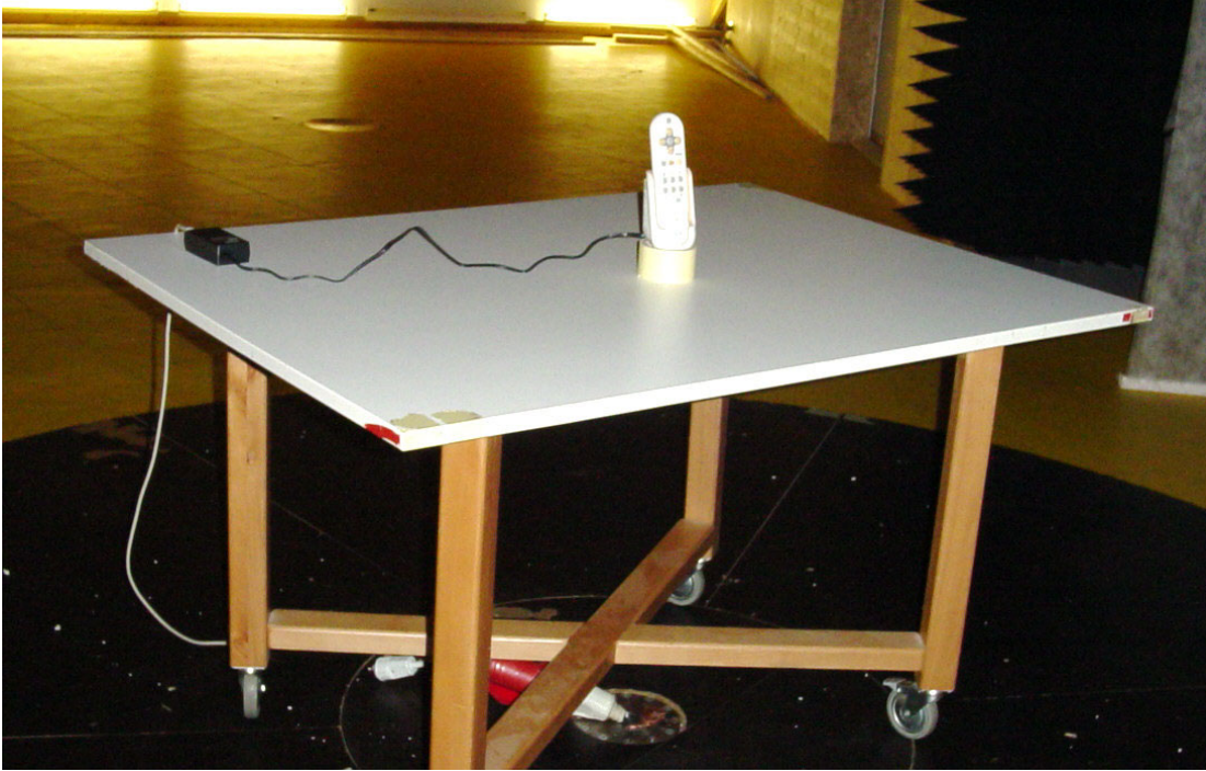
Radiated emissions test below 1 GHz; example set-up: emissions test in receive mode with charger
