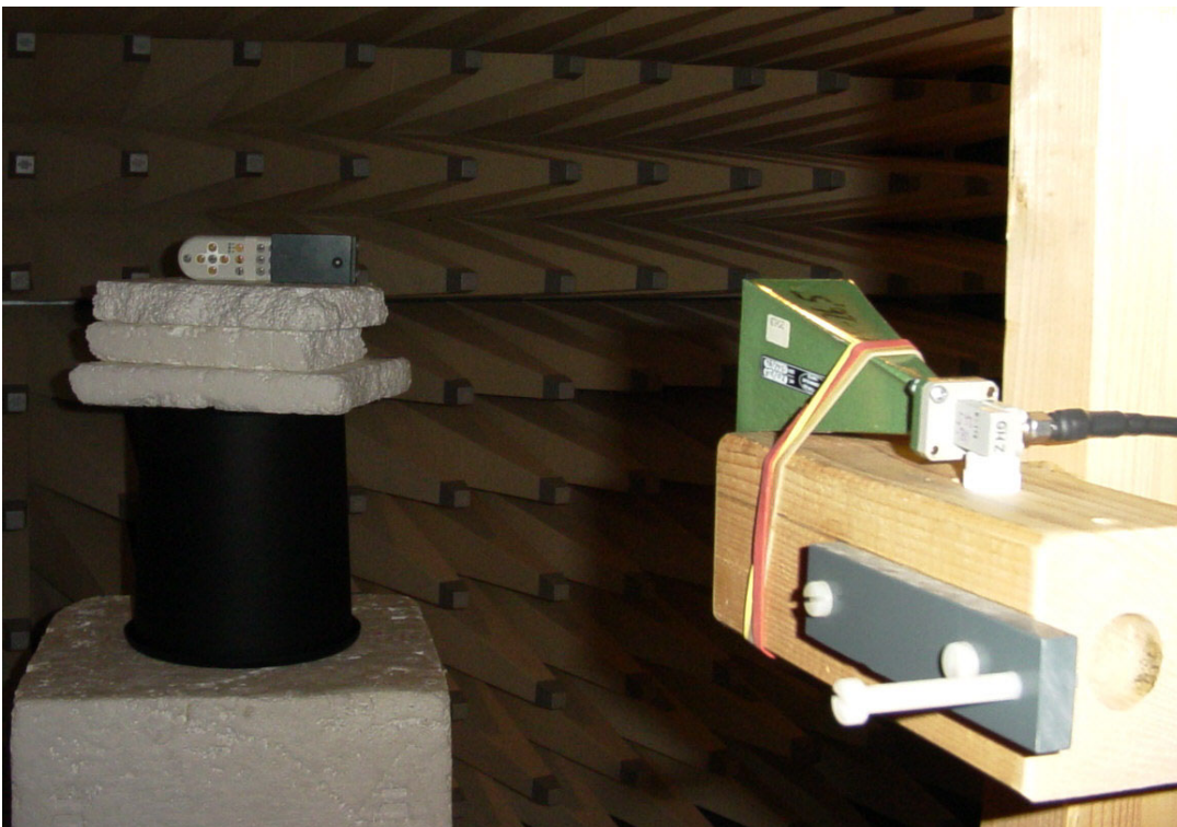
Radiated emissions test above 1 GHz; example set-up: emissions test 18 – 25 GHz
