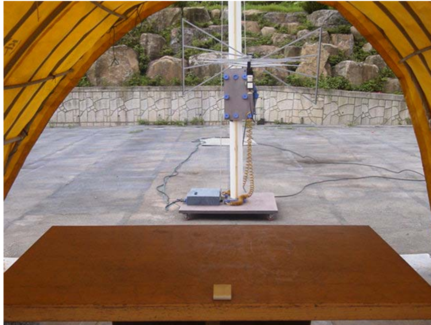
Photograph 1 : Setup for radiated Emissions
