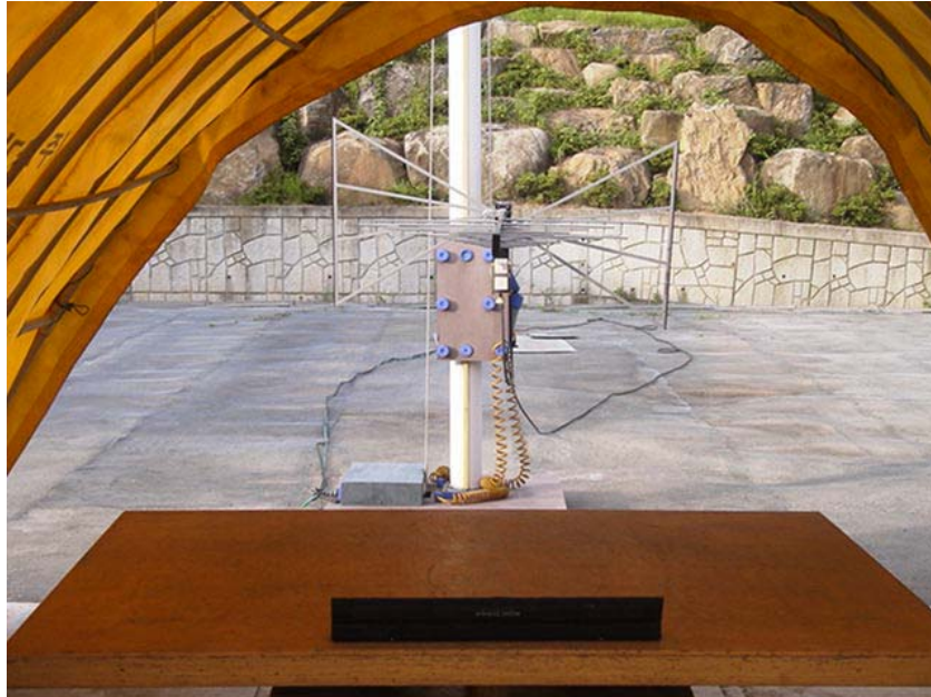
Photograph 1 : Setup for radiated Emissions
