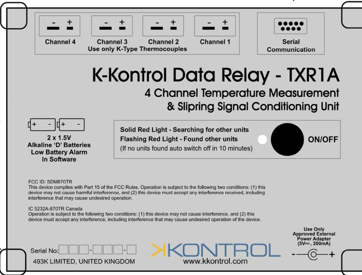
NOTES: DECAL ON BACK OF 250 MICRON LEXAN AND APPLIED TO ENCLOSURE WITH HIGH BOND STRENGTH ADHESIVE.
