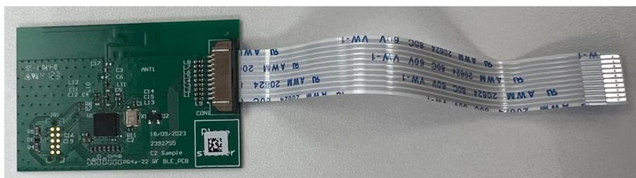
Connect the BLE-module with the flat cable.
