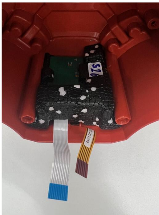
Connect the upper part with the BLE-module to lower housing part with the interface board
