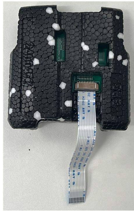
Mount the BLE-module holder in the upper part of the rotating laser housing
