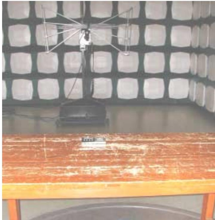
Measurement of Radiated Emission Test
