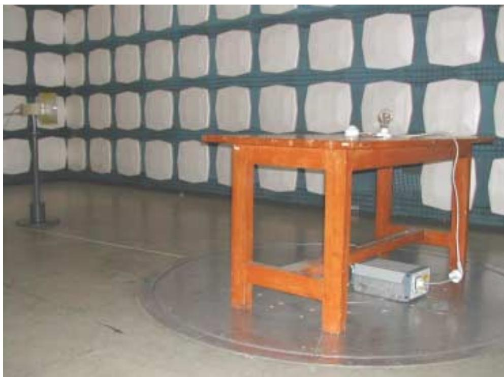
Measurement of Radiated Emission Test
