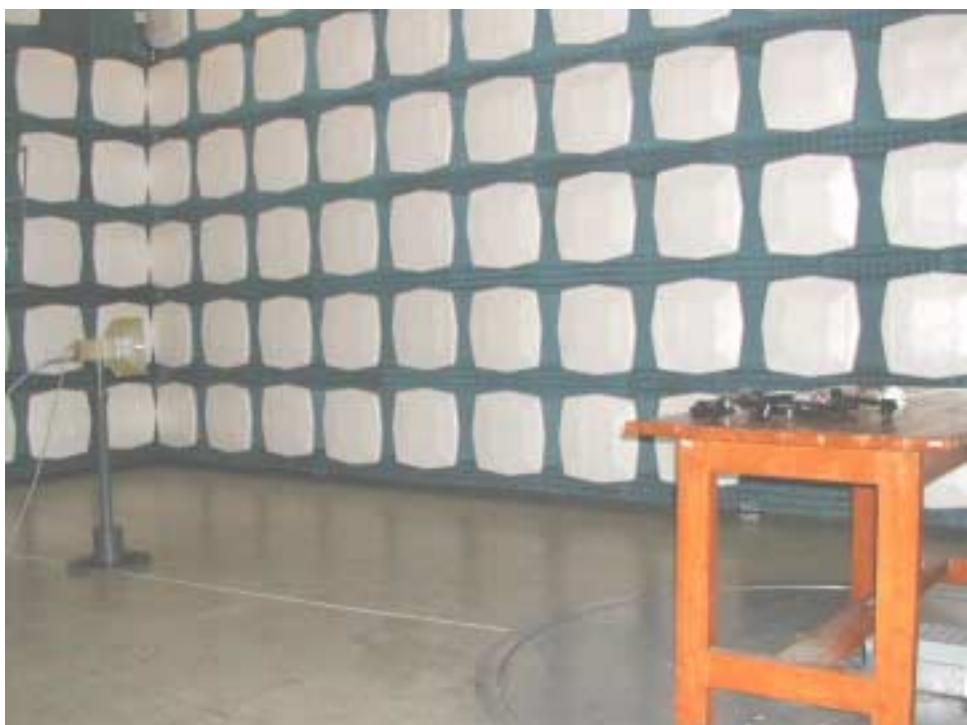
Measurement of Radiated Emission Test
