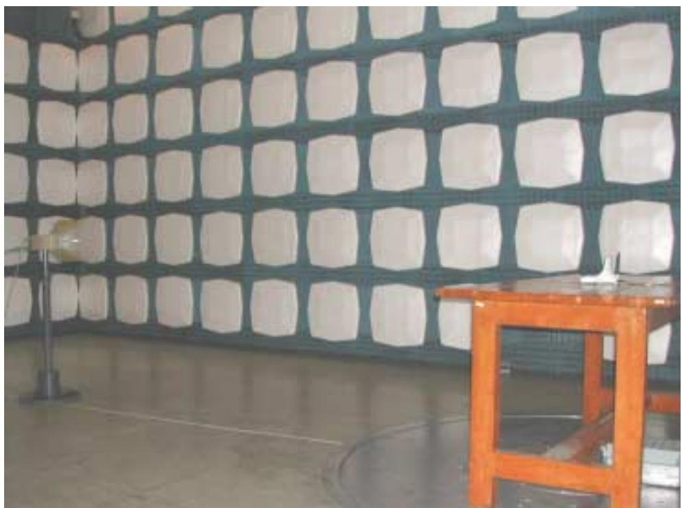
Measurement of Radiated Emission Test
