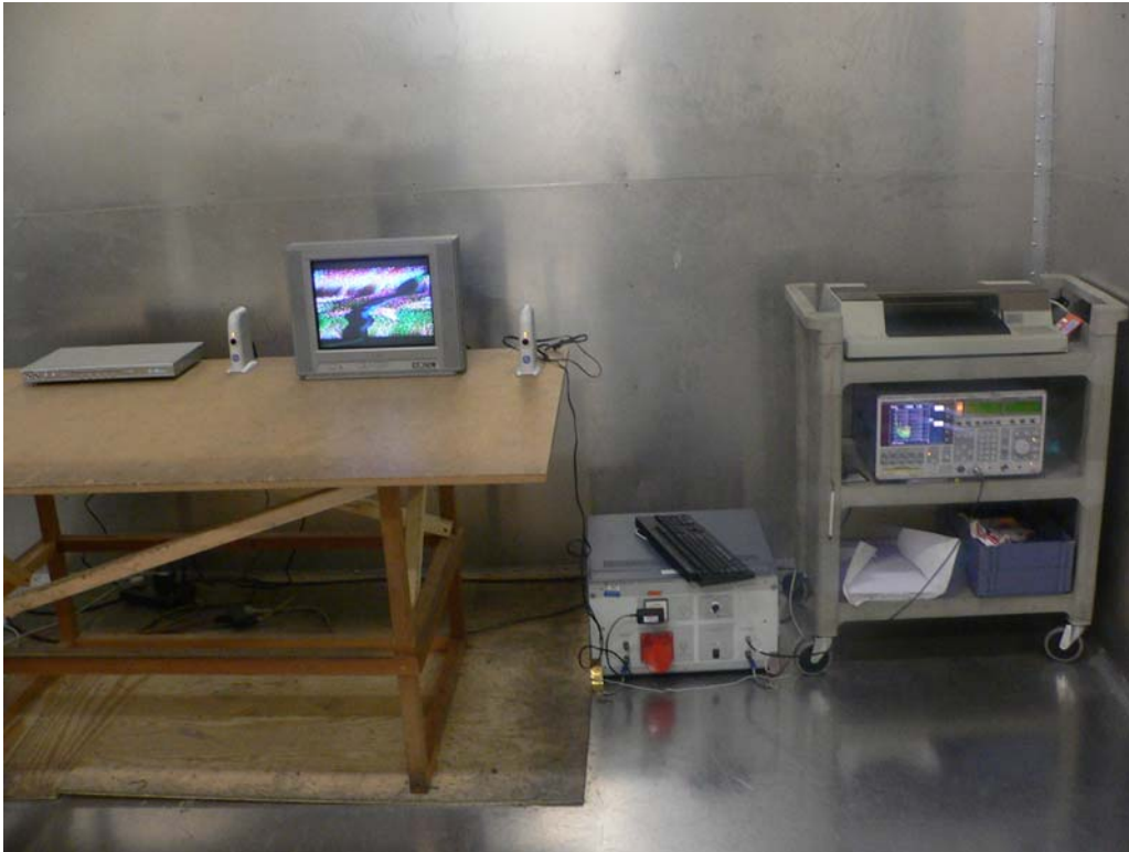
Conducted Emission – Front View
