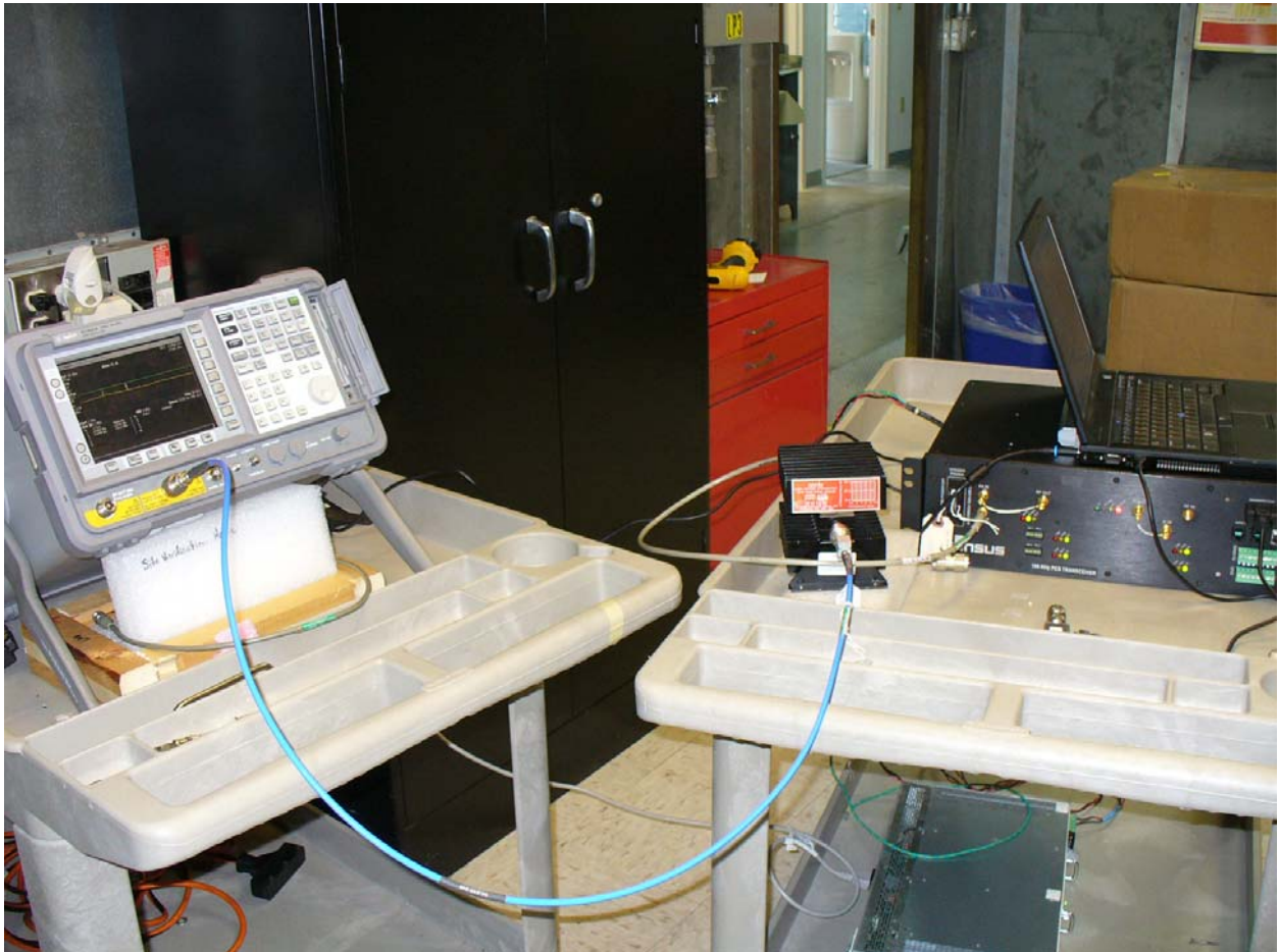
Figure 4: RF Conducted Emissions (Set Up 2)
