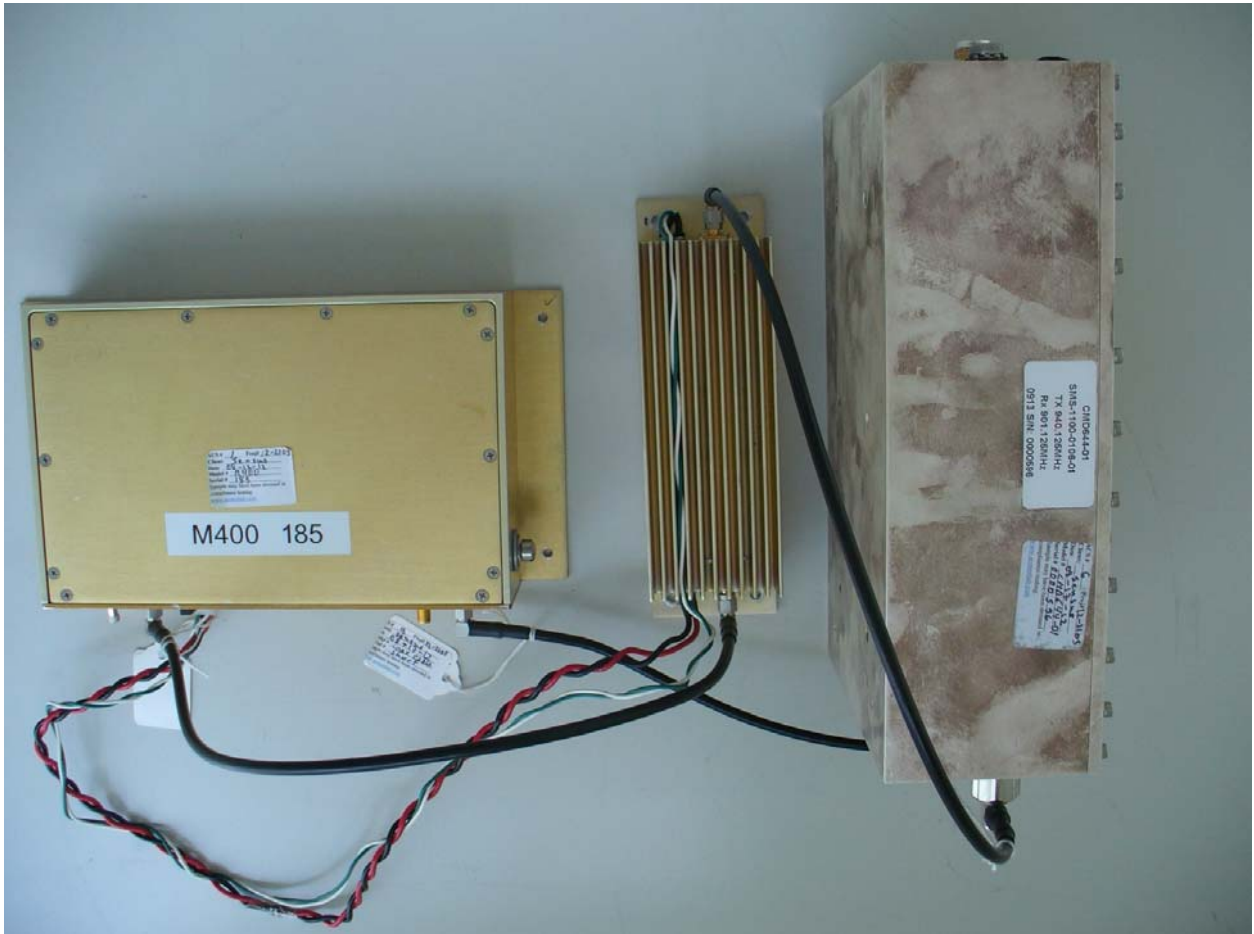
Figure 19: M400XCVR-01, Power Amplifier and Duplexer (Assembled – Top View)
