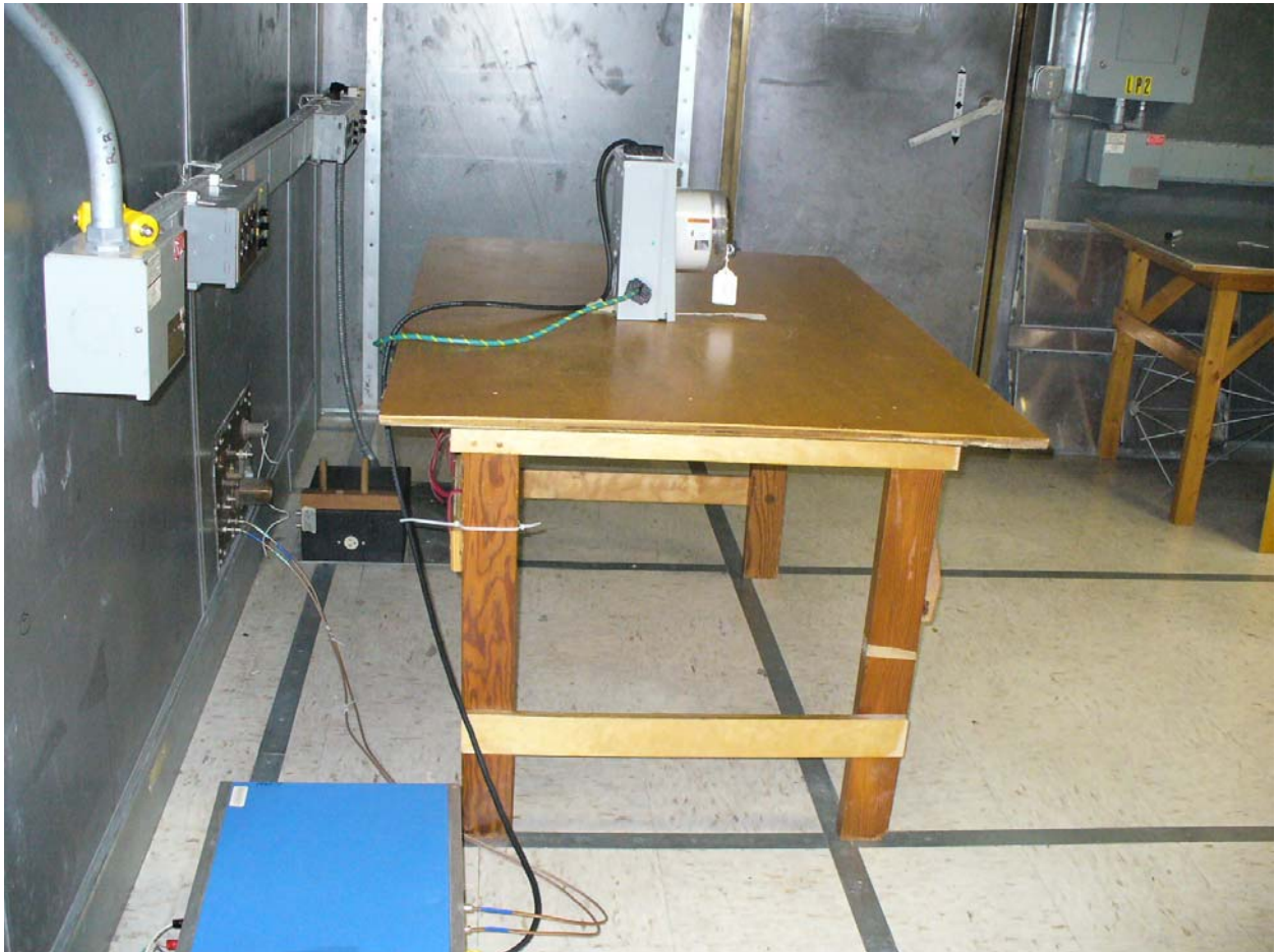
Figure 5: Powerline Conducted Emissions – Side View
