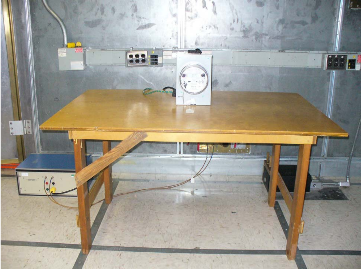
Figure 4: Powerline Conducted Emissions – Front View
