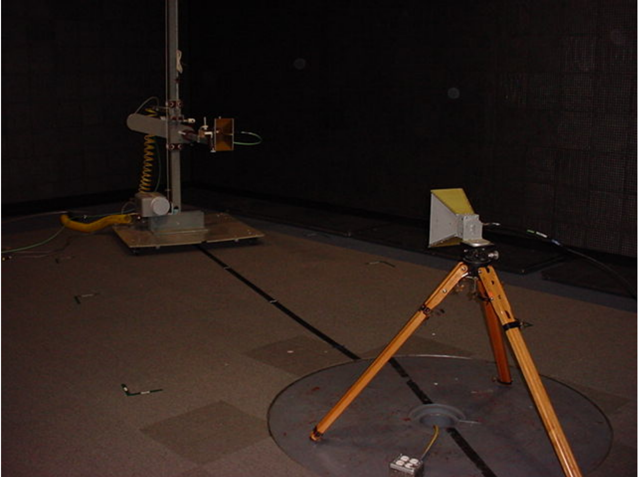
Figure 2: Spurious Emissions – Transmitter
