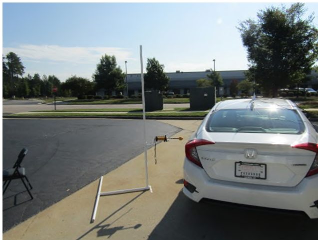
Photo 2.1.10-3 – Bystander at 60 degrees - Test Set-up
