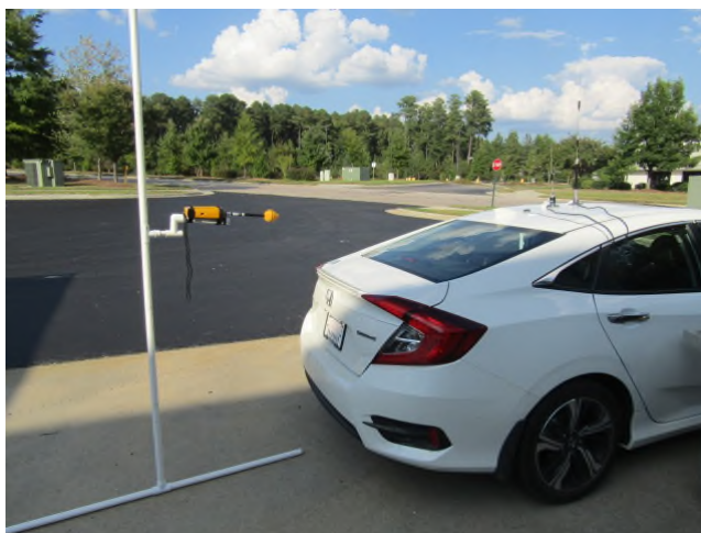
Photo 2.1.10-4 – Bystander at 90 degrees - Test Set-up
