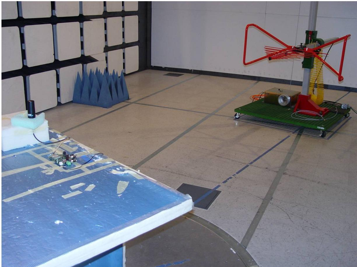
Radiated Emissions Module Test Configuration
