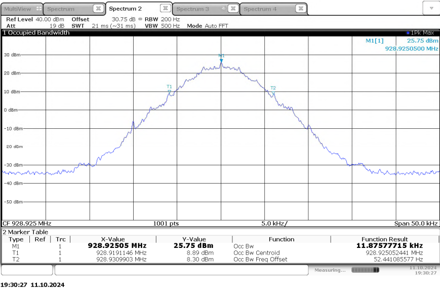
Figure 2.3.6-7 - 99% Bandwidth – TXC TCXO – 928.925 MHz - Normal Mode
