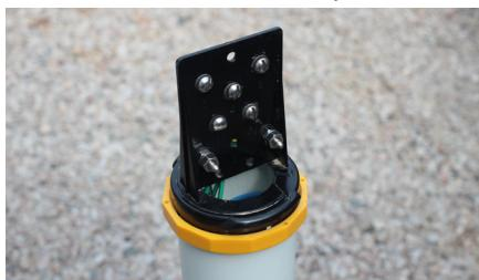
3. Carefully lift the test station up and away from the riser taking care not to damage the connected wires.
