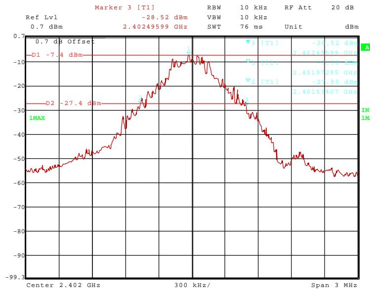
40450\_16.wmf (20 dB bandwidth at the middle of the assigned frequency band):
