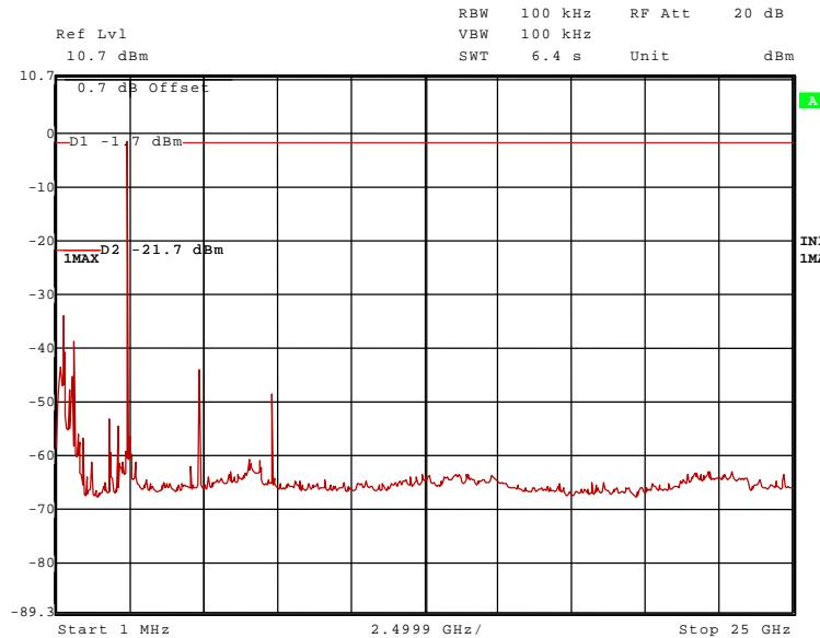
40450\_49.wmf (conducted emissions 1 MHz to 25 GHz, transmitter at 2480 MHz):
