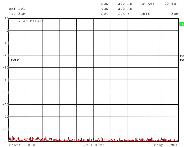
40450\_45.wmf (conducted emissions 9 kHz to 1 MHz, transmitter at 2441 MHz):
