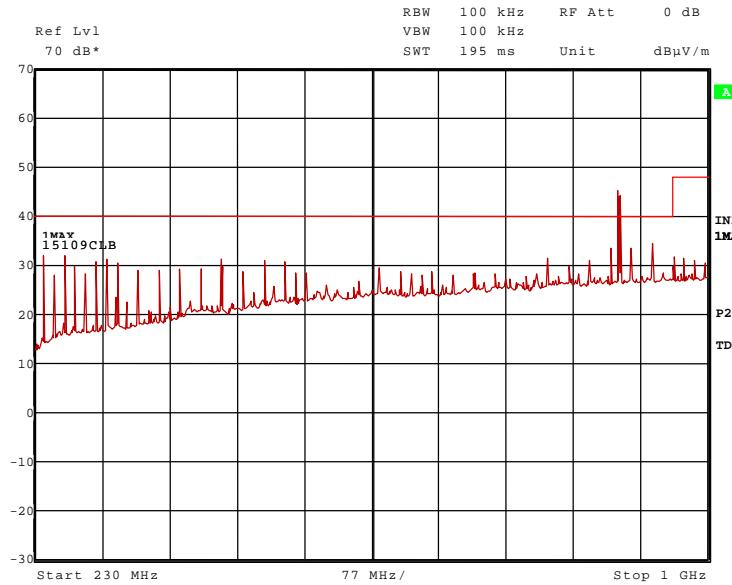
**Remark: The signal peak at 896.6 MHz, which lies above the limit line, is caused by a GSM mobile phone near the spectrum analyser and not by the EUT.**
