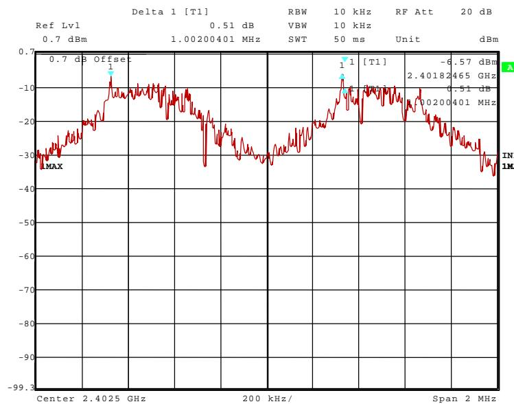
40450\_21.wmf (channel separation at the middle of the assigned frequency band):
