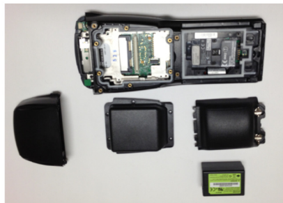
Psion Workabout Pro showing all inspection covers removed, battery removed and empty expansion bay.
