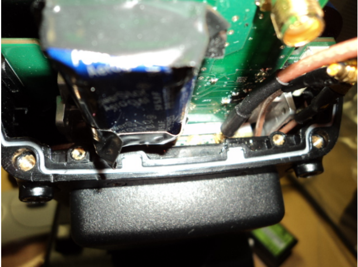
Figure 11: Other 900 MHz antenna ports investigated.
