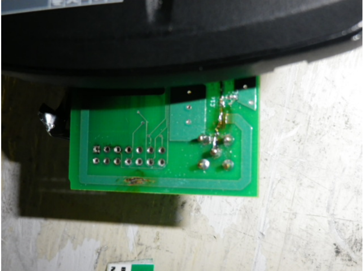
Figure 10: Antenna Modification: 433MHz antenna cut from circuit for conducted measurements.
