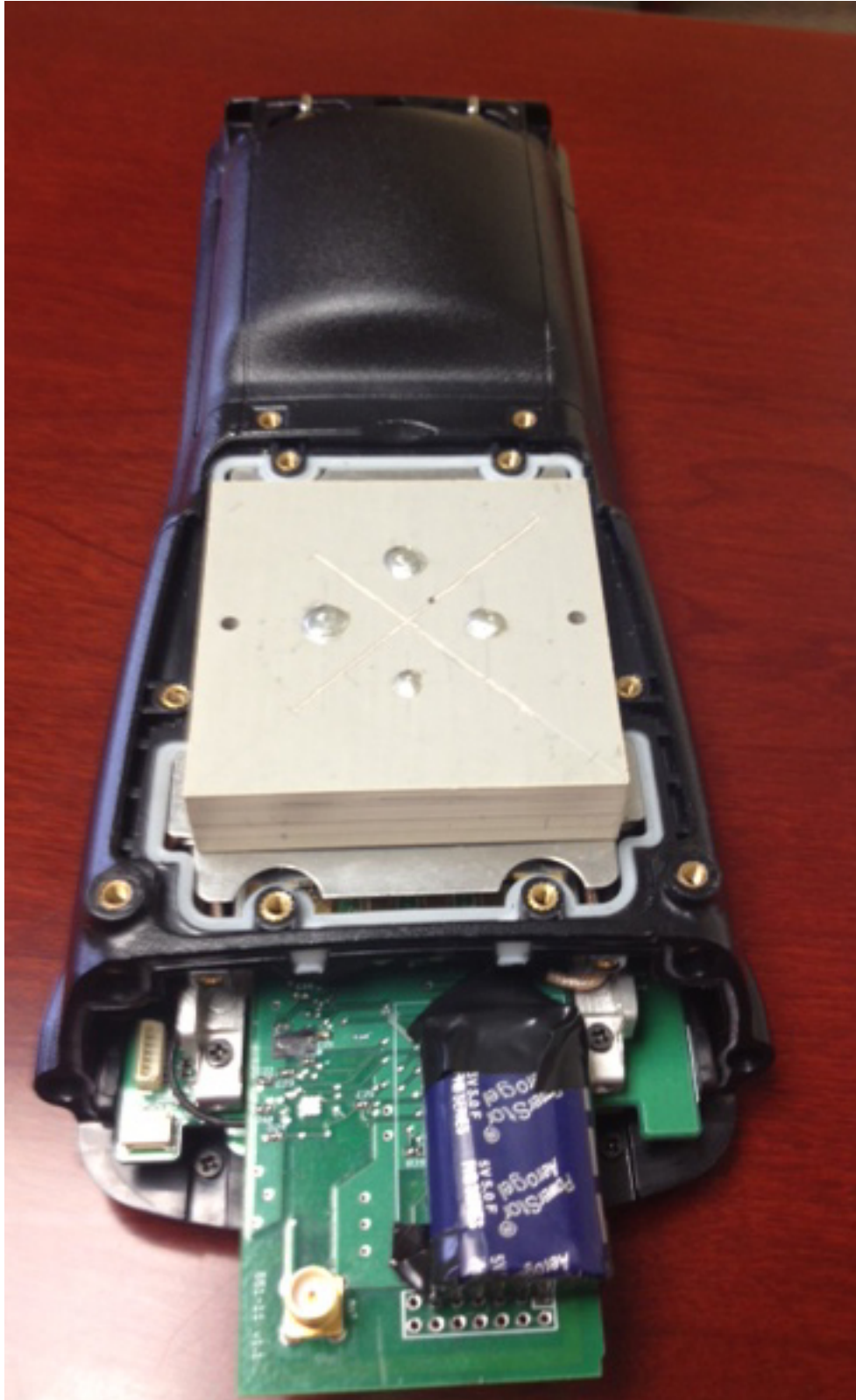
Figure 4: Location of 900 MHz multi-antenna package
