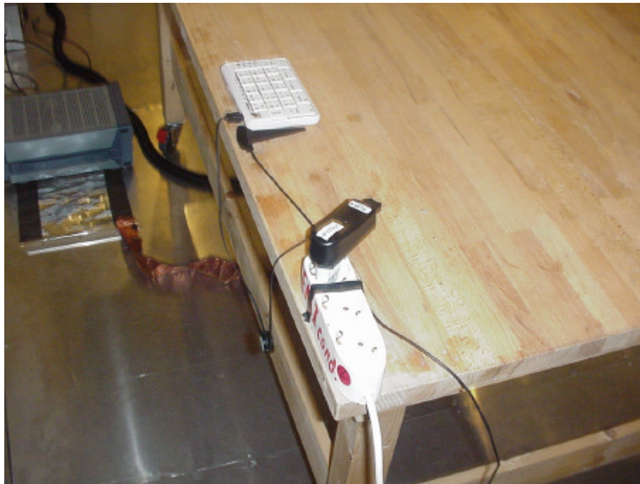
Picture 1 : Setup for conducted emissions tests
