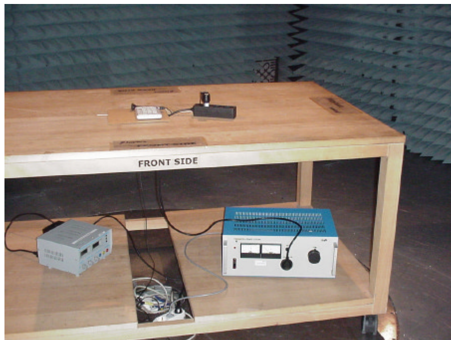
Picture 2 : Setup for radiated emissions tests
