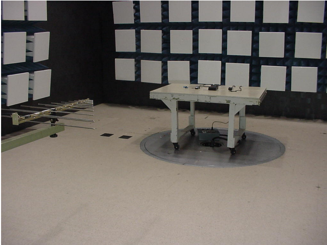
Figure 2 - Radiated Emissions Test Setup (Chamber - Front)
