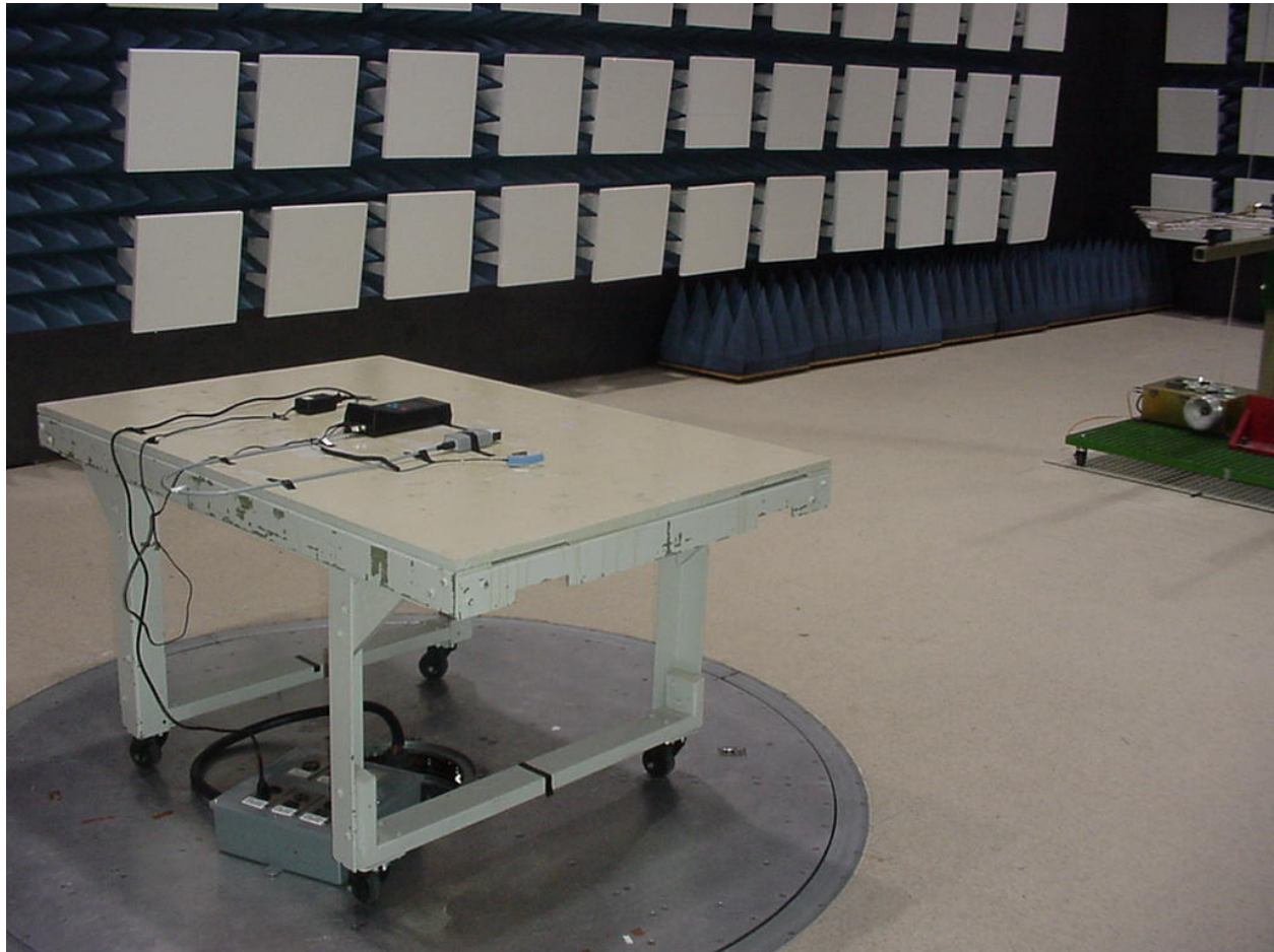
Figure 3 - Radiated Emissions Test Setup (Chamber – Back)
