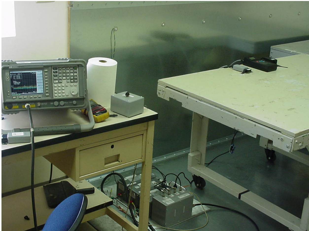
Figure 4 - Conducted Emissions Test Setup (Front)
