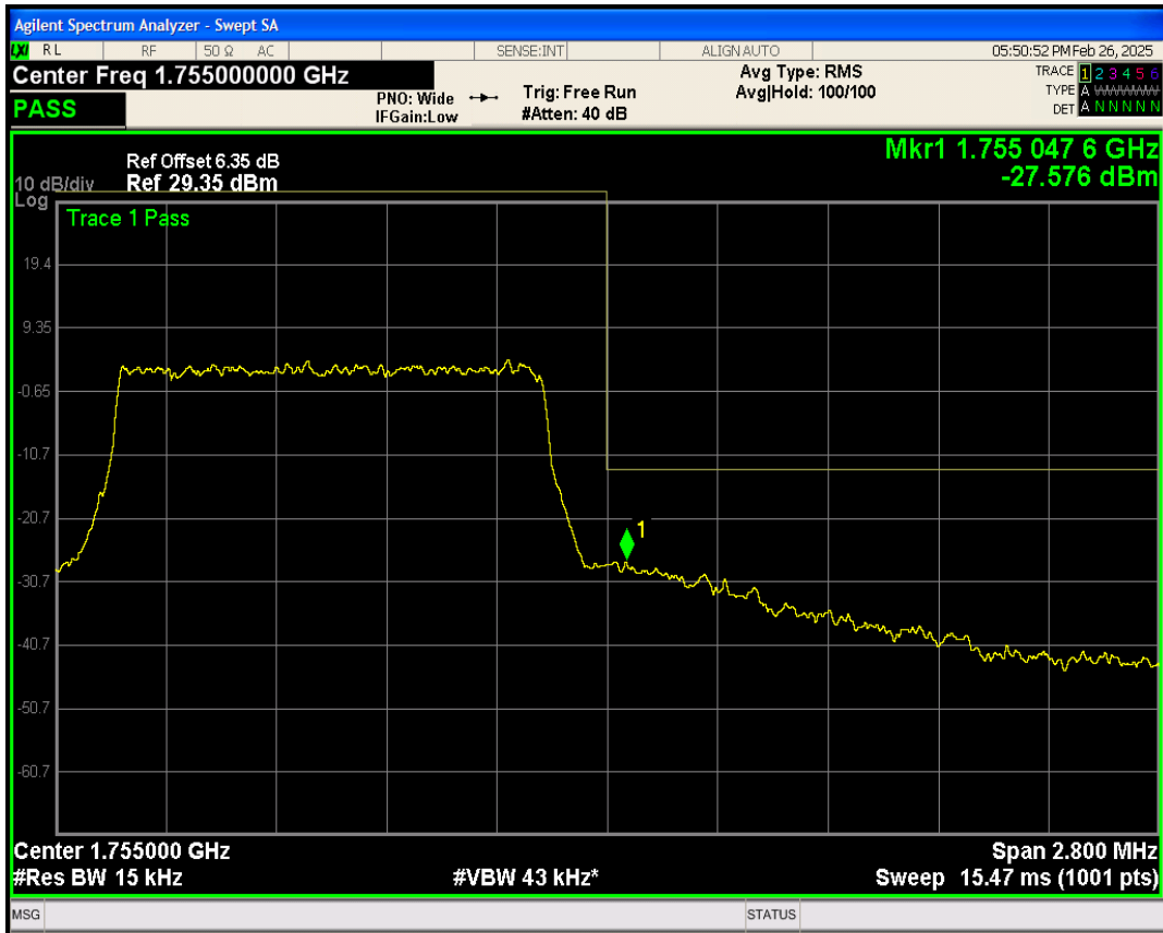
Band4 16QAM BW=1.4MHz Channel=20393 RB Size=6 Position=#0
