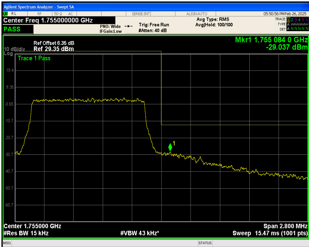
Band4 QPSK BW=3MHz Channel=19965 RB Size=15 Position=#0
