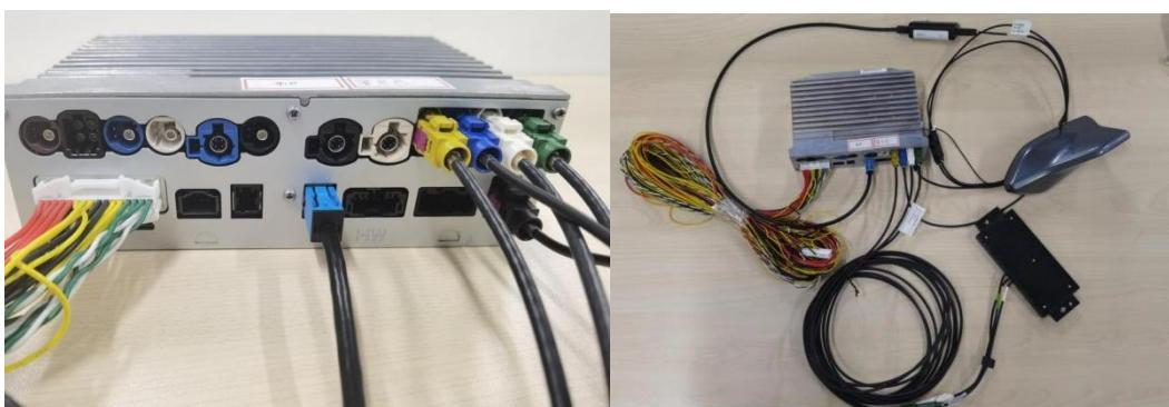
M1 interface host power line, the harness can be modified according to requirements, in which red and black lines are mainly used, red is connected to the positive pole, black is connected to the negative pole, and other lines are can lines, which do not need to be connected.
