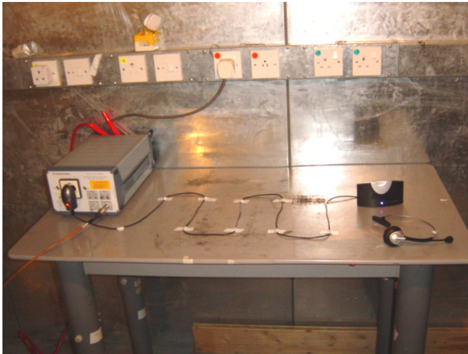
Set-up for AC mains conducted Emission (operating mode)
