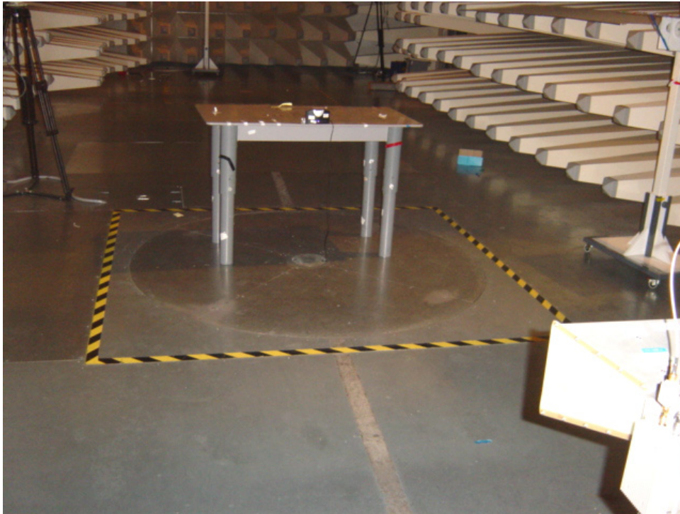
Set-up for Radiation Emission (Transceiver)
