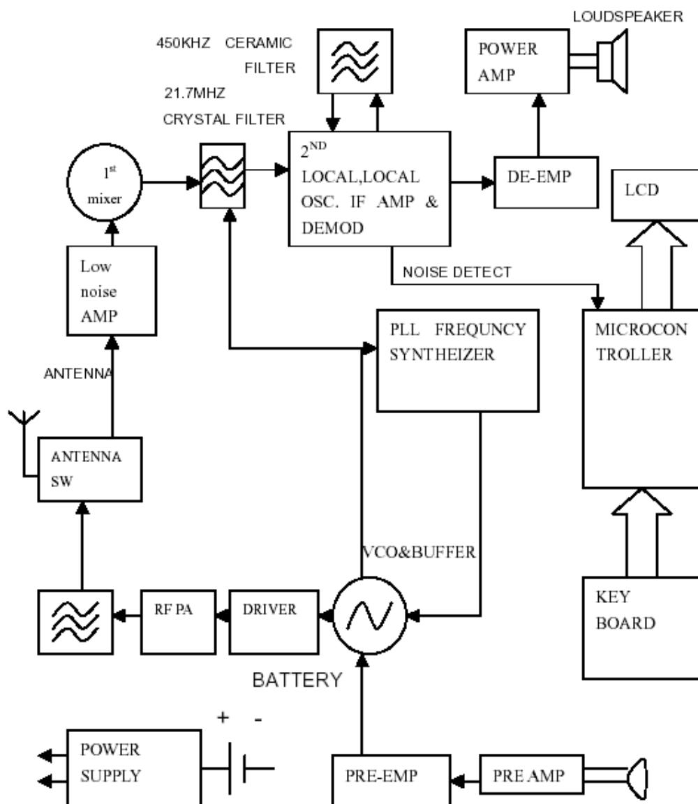
As is evident in the above block diagram, this product employs dual-conversion superhet architecture for its receiver. The first IF (Intermediate Frequency) is 21.7MHz. The second IF is 450kHz. The local oscillator signal is PLL-synthesized to ensure accuracy and stability. A microcontroller with appropriate firmware is designed to program the PLL to the desirable user-selected channel for either transmit or receive.
