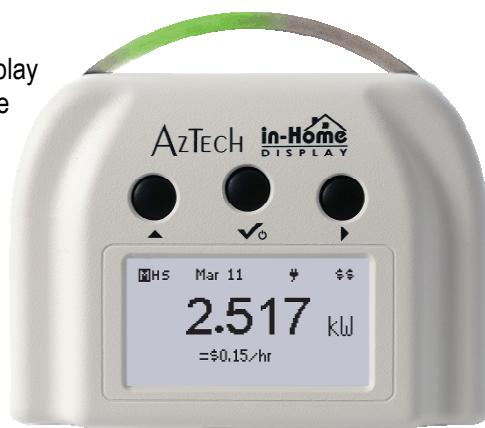
When the AC power adapter is connected, the Indicator Light Bar sweeps continuously. When operating on batteries, the Indicator Light Bar normally stays off to conserve battery power. It turns on for a short duration when changing display screens or when the buttons are pressed.
