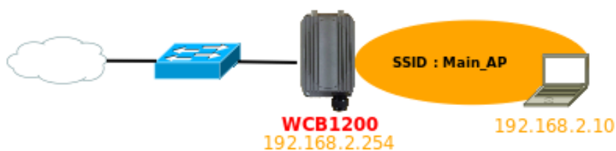
Figure 3-1 Access Point on a Wired LAN Configuration
