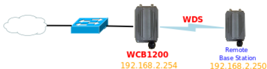
Figure 4-1 Point to Point network Configuration
