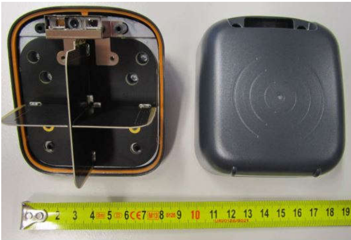
Cross dipole antenna front view
