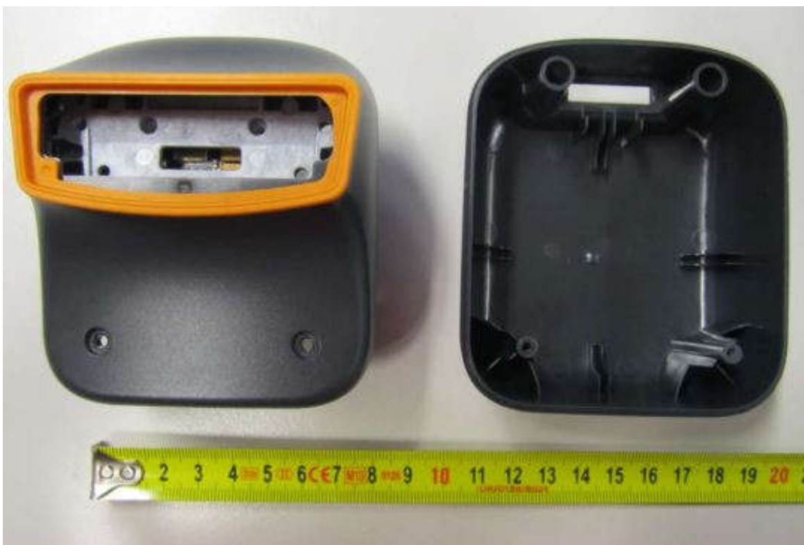
Cross dipole antenna covers and connection to host product
