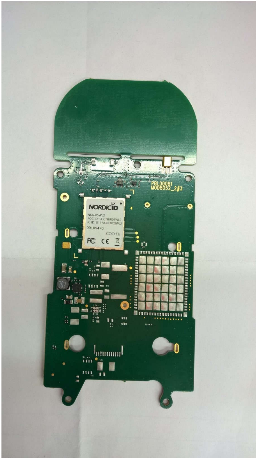
Picture 14. Merlin 805-2C MOD board top.
