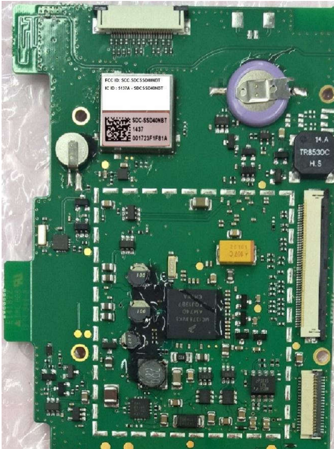
Picture 12. SDC-SSD40NBT module in Merlin CD 805-2C main board.
