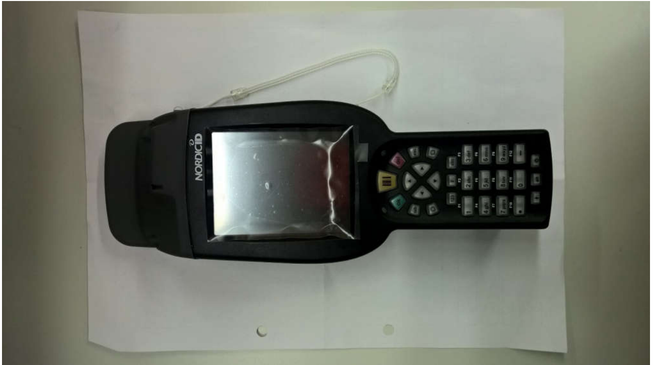
Picture 1. Merlin 805-2C front side. Length X Width X Height=254mm(L) X 91mm(W) X 49mm(H)
