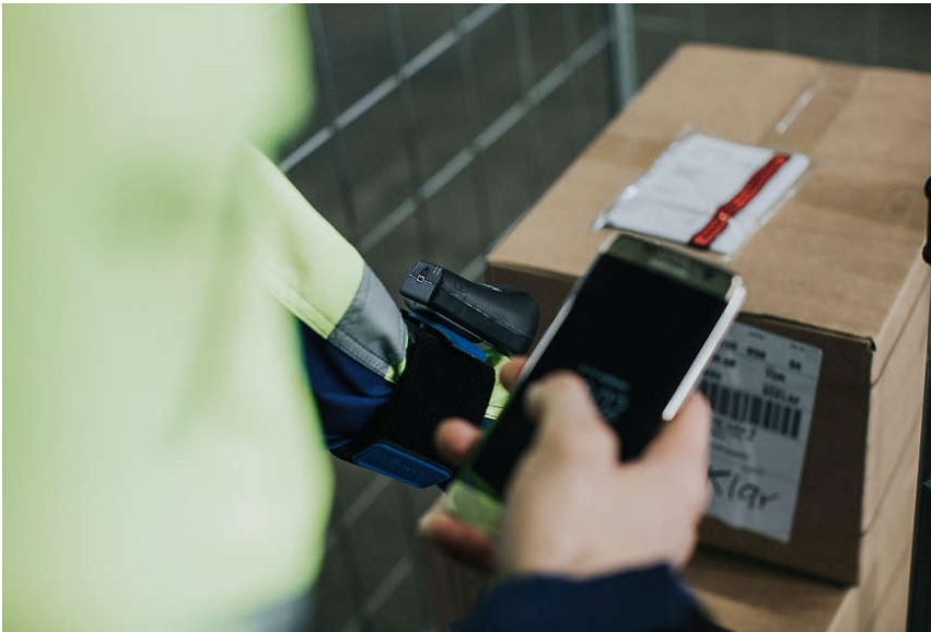
EXA31 mounted into arm with wrist band + quad lock. Smartphone is used to display information from Barcode / RFID tag.
