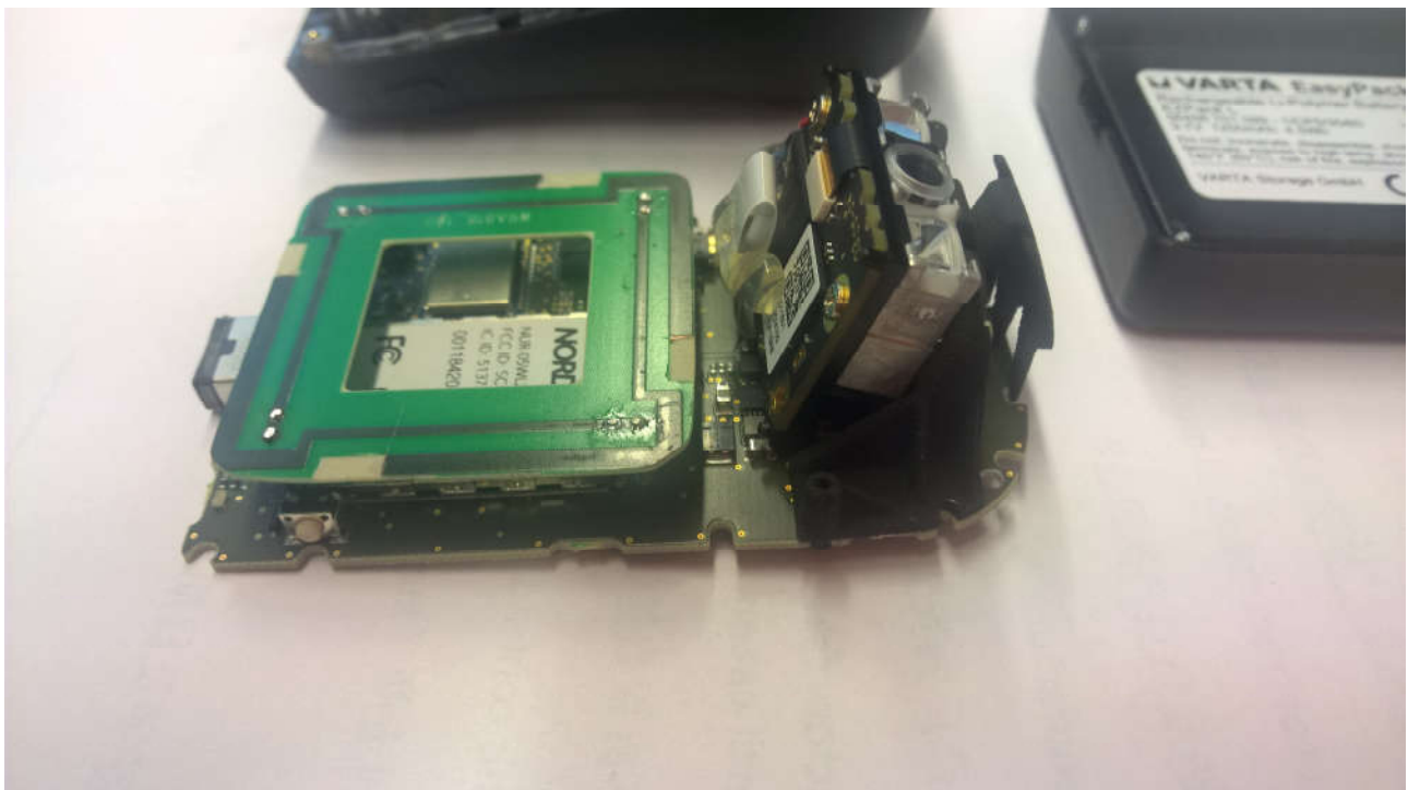
Pic. 4: EXA31 with 2D imager for barcode reading.
