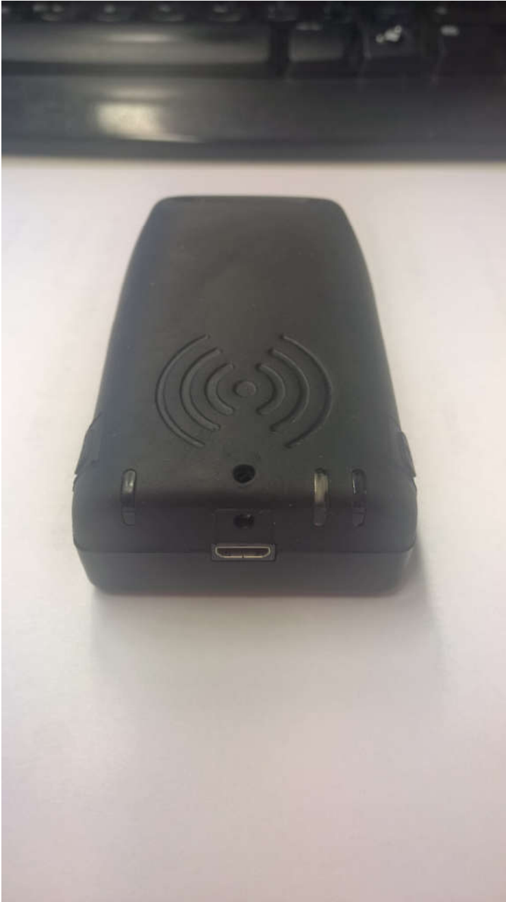
Pic. 9: EXA31 USB connector & LED's.
