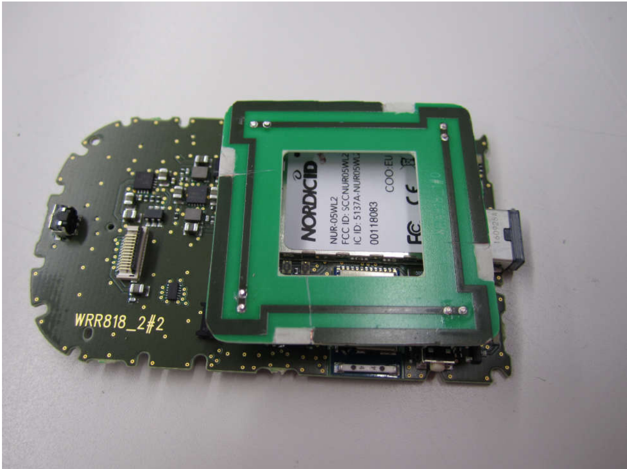
Pic.3: EXA31 with RFID antenna installed
