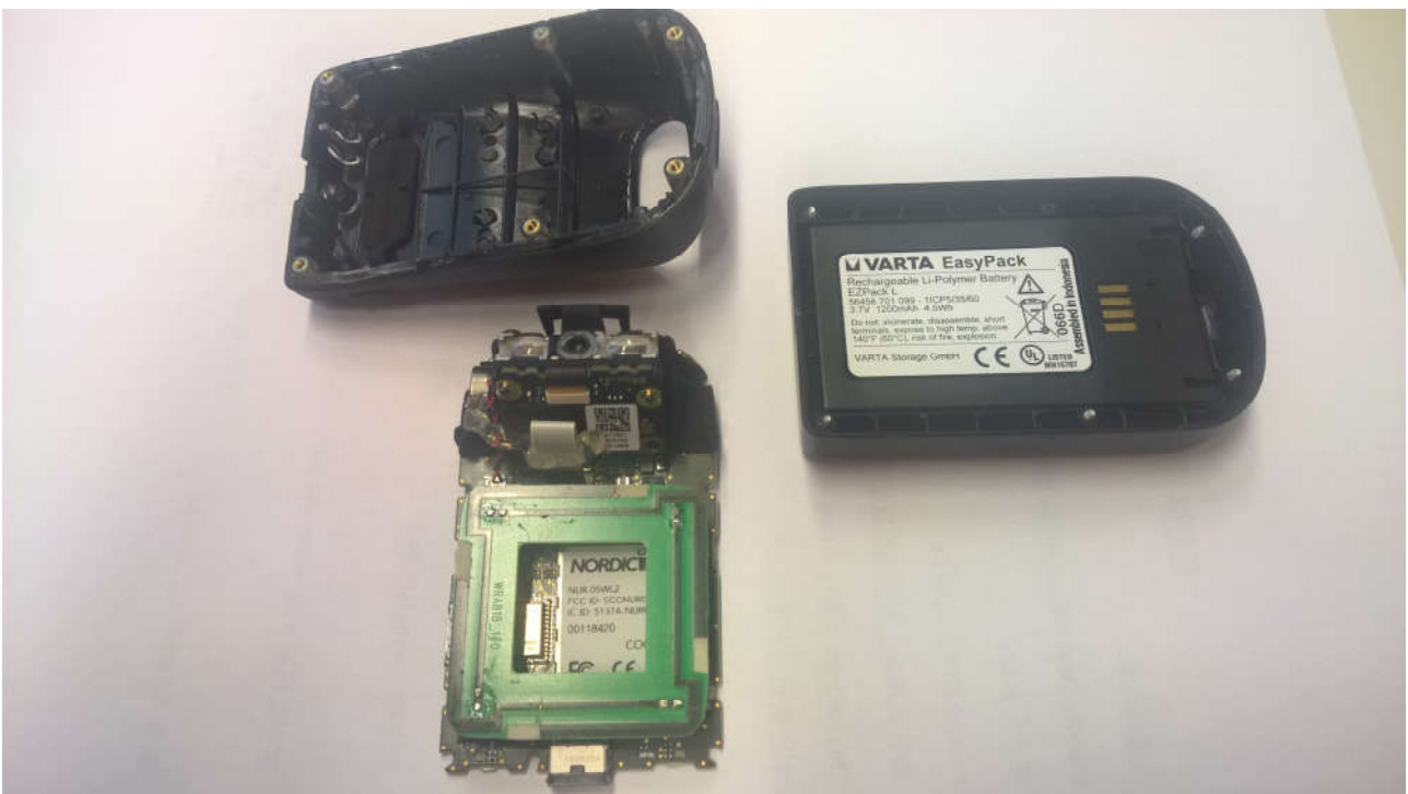
Pic. 6: EXA31 with 2D imager for barcode reading.
