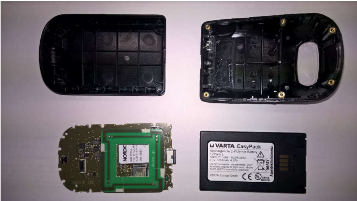
Pic. 5: EXA31 A+B covers, CPU board and battery
