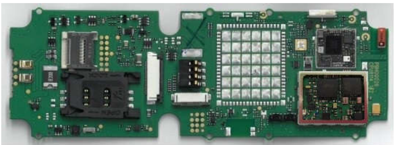
Picture 4: CPU811 board bottom side without NUR-05WL2 and SSD40NBT shield
