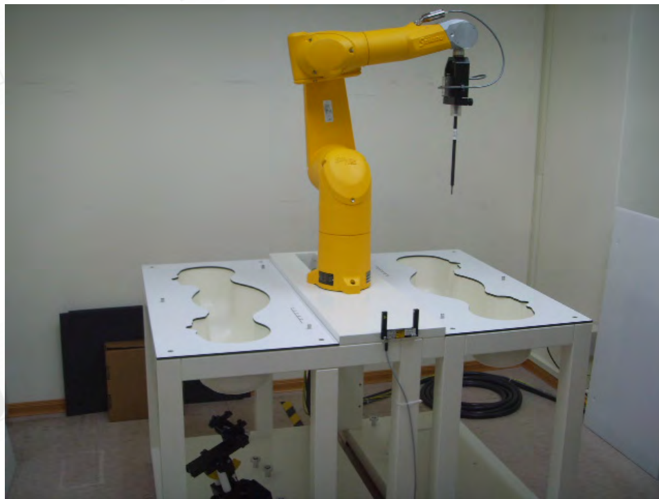
Fig.1 Photograph of the SAR measurement system
