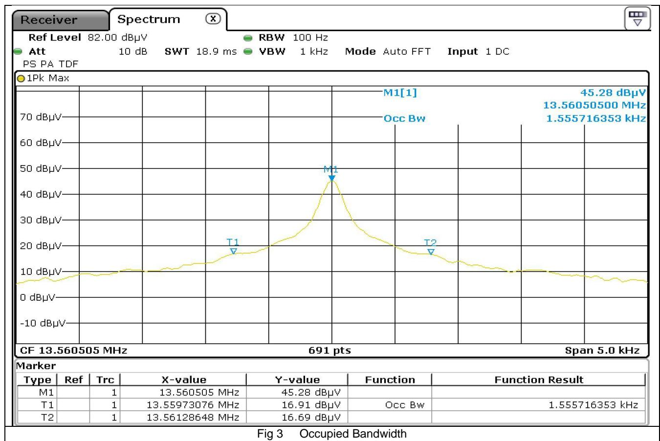
13.56MHz Occupied Bandwidth = 1.56KHz
