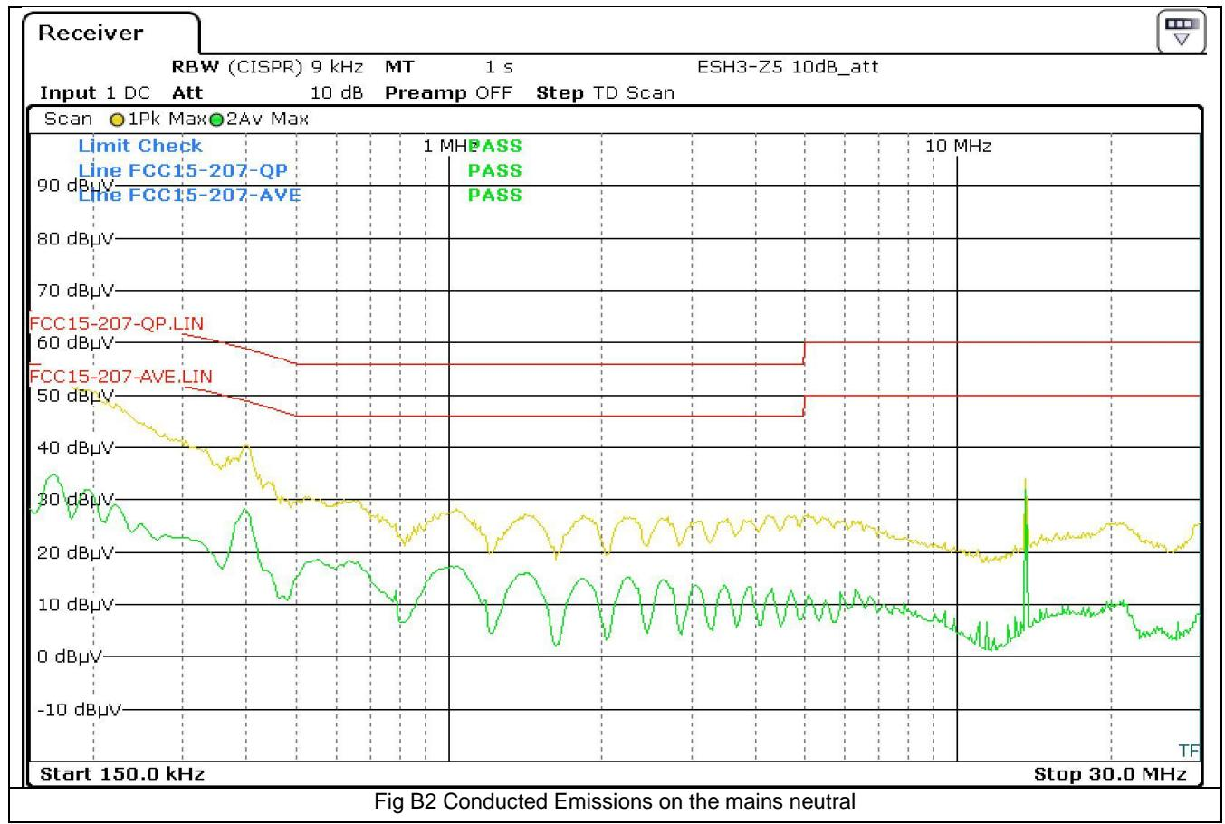
Fig B2 Conducted Emissions on the mains neutral
