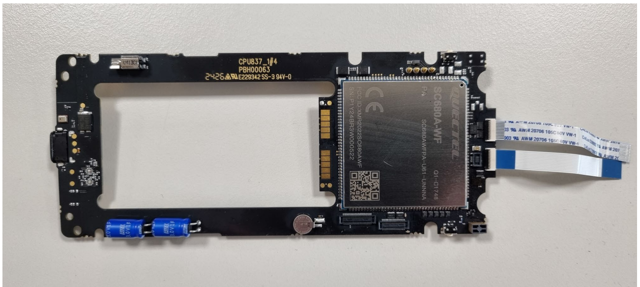
Picture 4. HH86 main unit PWB top. WLAN + BT/BLE module SC680AWF visible
