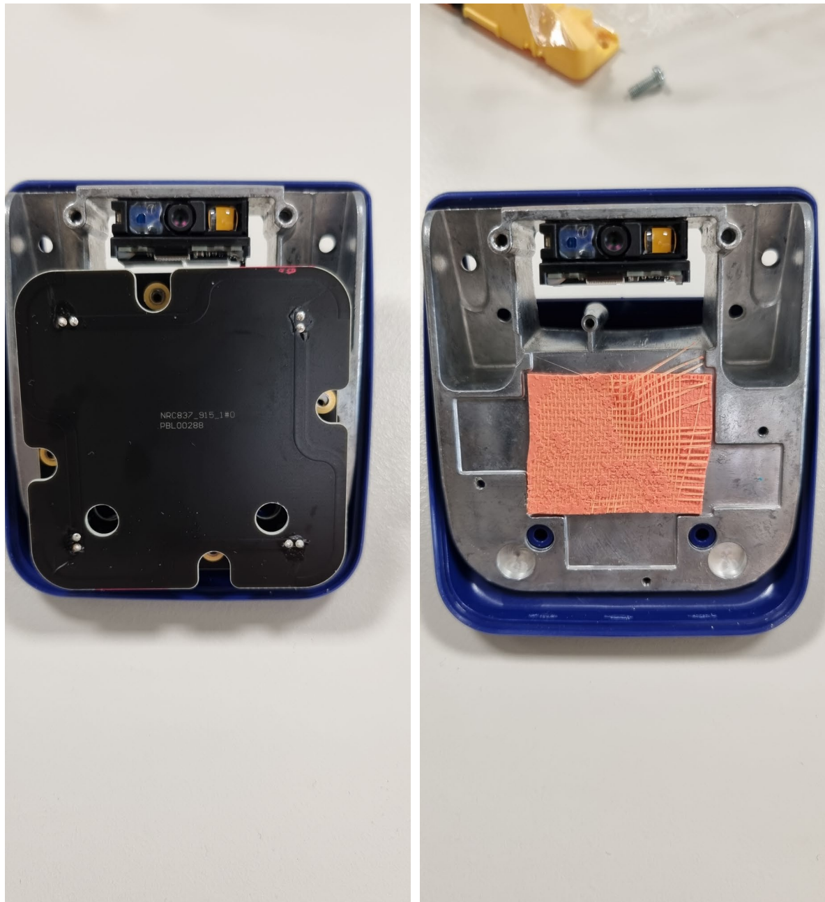
Picture 9. HH86 RFID module + antenna mounted into the HH86 RFID front end unit.
