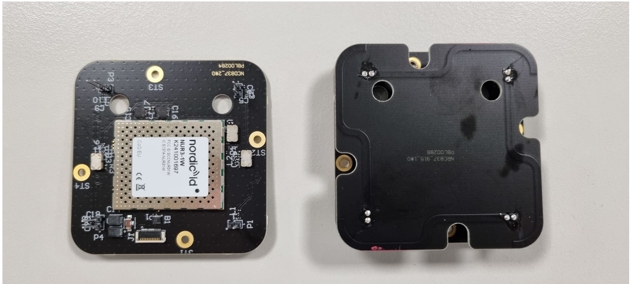
Picture 7. HH86 RFID module in left and module + antenna mounted at the top of the module in right photo.
