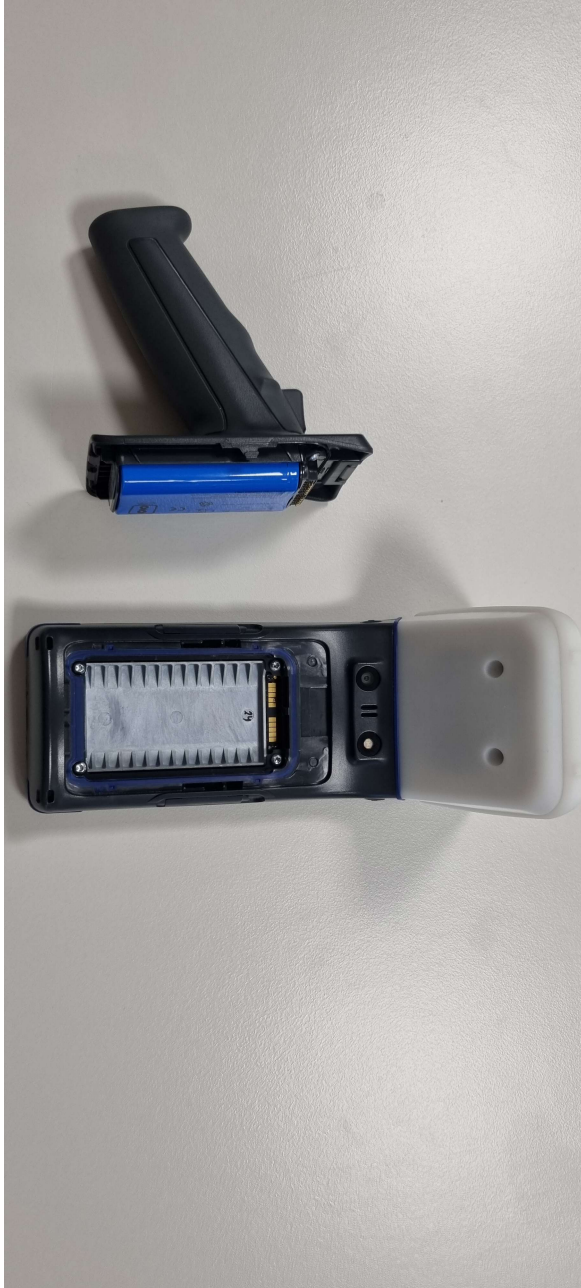
Picture 9. HH86 Brady HH86 pistol grip detached.
