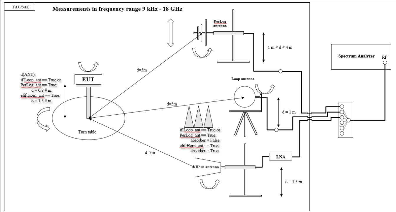
\* depending on limit line different horn antennas, correspondingly different measurement distances, can be used.
