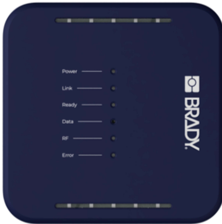
Picture 2 The placement of individual LEDs and the LED bars of the Brady IRX200
