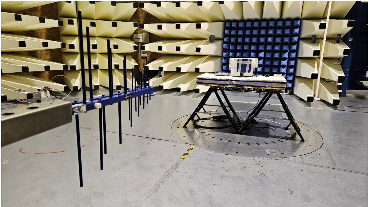
Radiated Emissions 300MHz-1GHz test with external antenna
