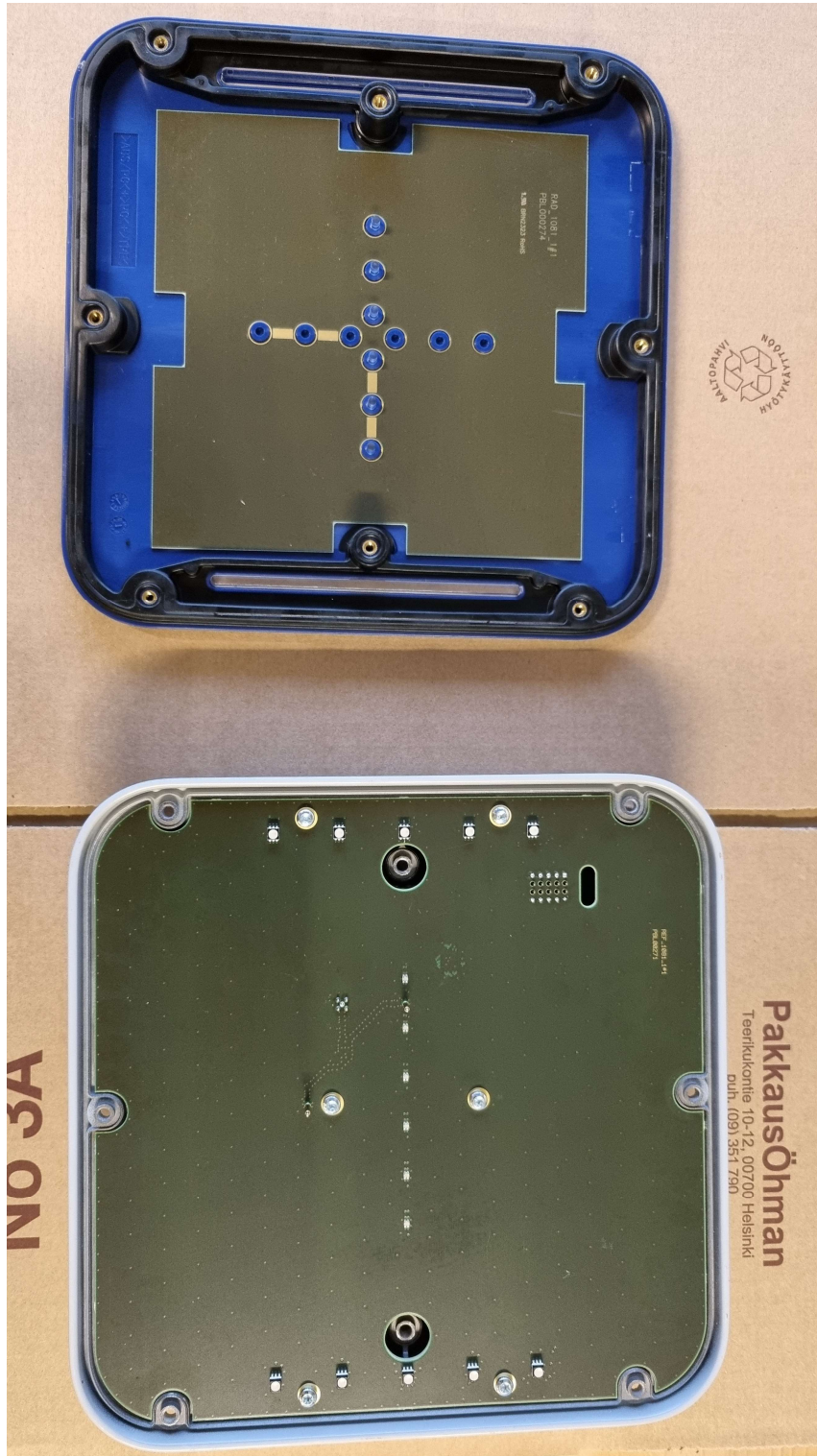
Picture 1. A cover disassembled from B cover. Antenna reflector attached into blue A cover.
