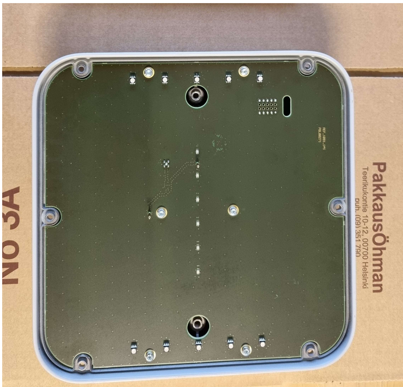
Picture 2. IRX200 RFID Antenna radiator top side in B cover.
