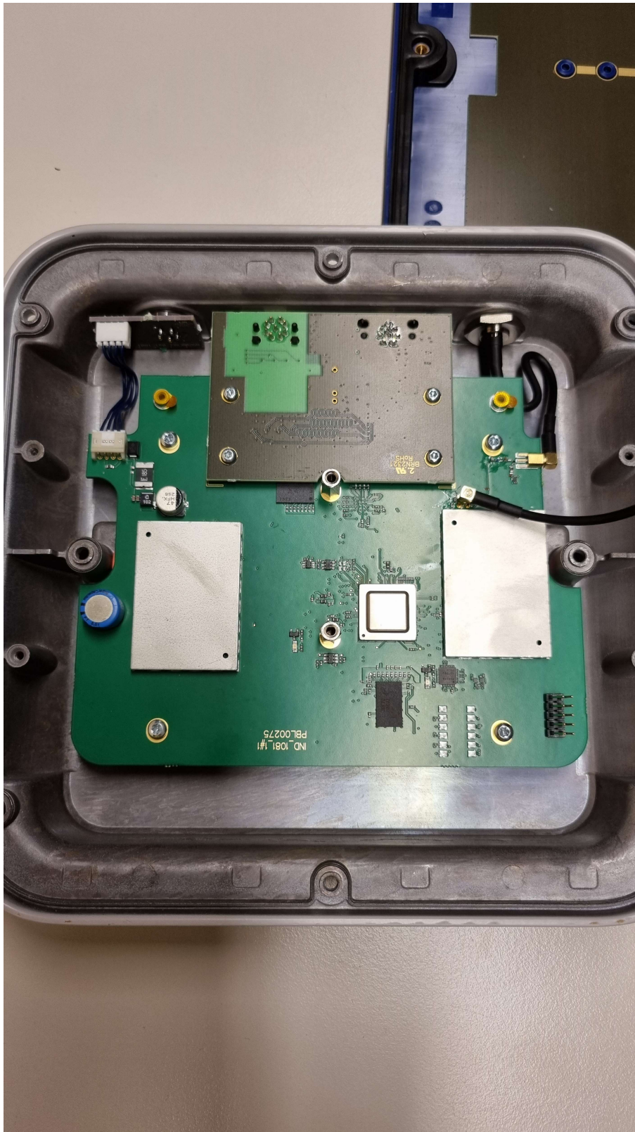
Picture 3. IRX200 main PWB top side including RFID and supporting electronics.
